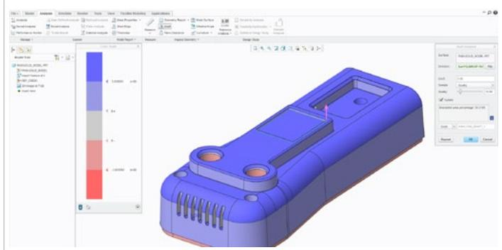
**New connection analysis tools:** PTC Creo Parametric introduces a new connection analysis tool to analyze position, tangency, and curvature continuity of curve and surface connections. Rather than select individual surface boundaries and curves, the user is able to quickly analyze the entire model to highlight connections that do not meet the design criteria.
