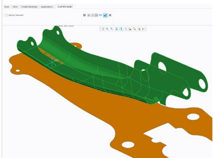
**Advanced support for patterns:** Geometry pattern capability has been extended in PTC Creo Parametric to allow users to pattern geometry across an area of topology change. This significantly improves the usage of geometry pattern and significantly improves overall productivity. In addition users can now reference pattern features that have been placed on any pattern instance, rather than needing to always place the features on the references of the pattern leader.
