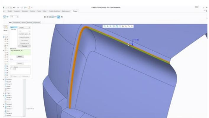
**Sheetmetal productivity:** Rapidly create sheetmetal geometry using new functionality to automatically apply bend relief, create sheetmetal rips, bend coplanar geometry, and simplify die form and flat pattern creation.
